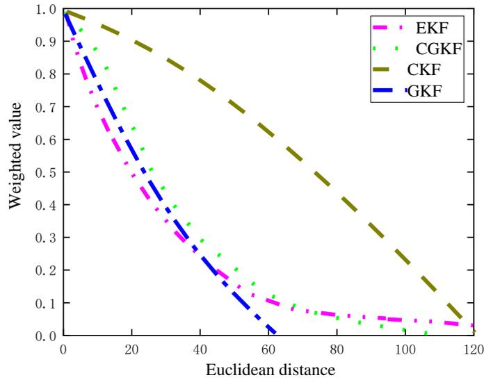
Figure 1. Response curve of weighted kernel function
