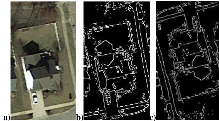
Figure 6. a) Image before Canny Edge Algorithm; b) Image after Canny Edge Algorithm; c) Image after Canny Edge Algorithm and Augmentation
