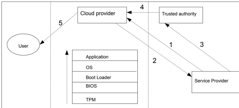
FIGURE 1 – Architecture of the proposed trusted SaaS platform
