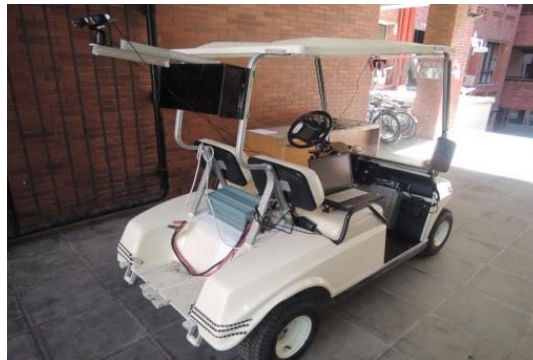
Figure 7. The golf cart with stereo vision for actual parking experiments
