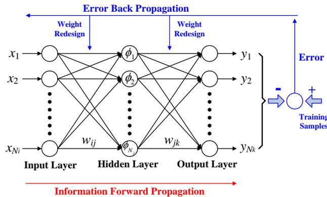
Figure 1. Topology structure of a BP neural network.
