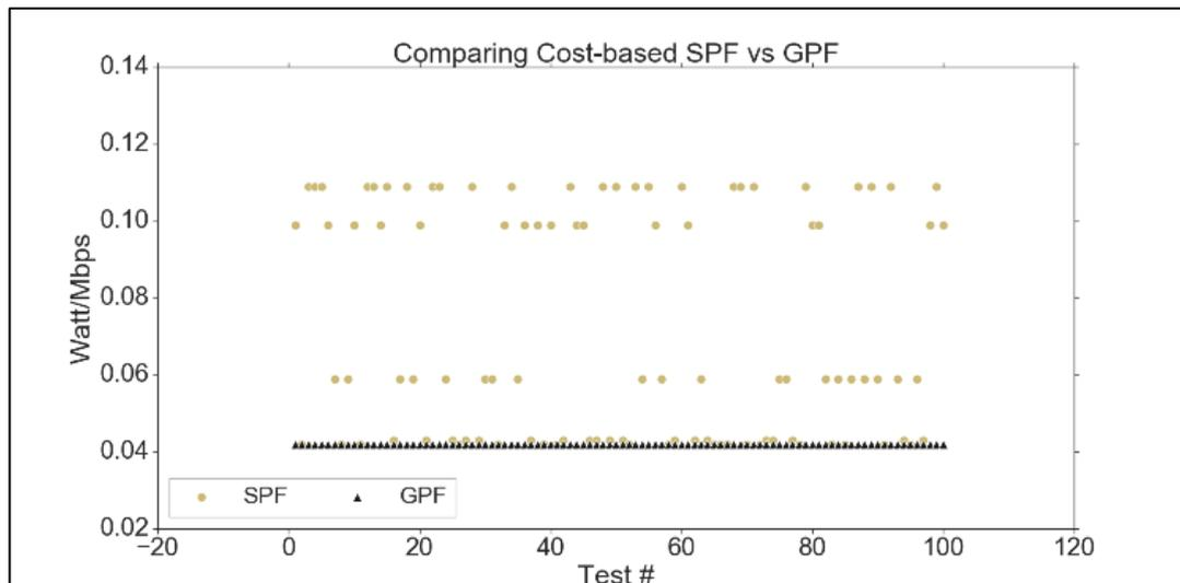
Figure 5. Comparing Watt/Mbps - cost-based SPF vs GPF
