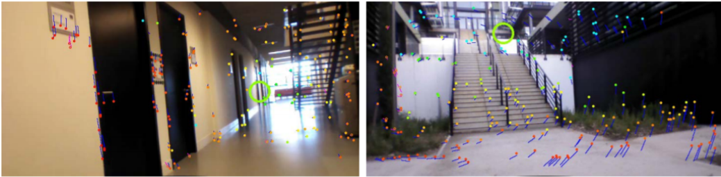
Fig. 2. Sparse3D indoor (left figure) and outdoor (right figure) reconstruction based on a few dozens of points. Blue/purple lines show optical flow vectors consistent/ conflicting with the camera's motion. The points in color represent their longitudinal distance – red indicates 1 meter or less, cyan for 10 meters or more. A larger green circle marks the flight direction targeted by the drone, which is computed according to the furthest possible distance with no potential obstacles
