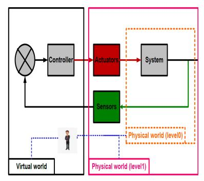
Figure 7. Closed-loop model of a CPS
