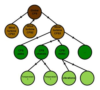
Figure 10. Tree diagram of a CPS
