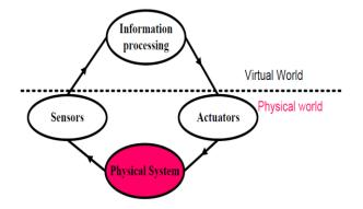
Figure 2. Principles of Cyber-Physical Systems operation
