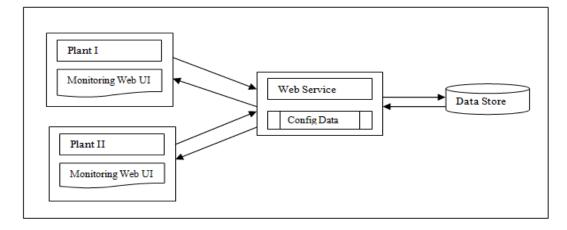
Figure-2 shows the design of the application after it was modified for migration to cloud.
