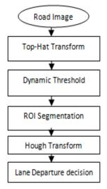
Figure 3. Flow of the algorithm
