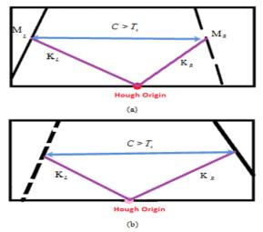
Figure 5. New Lane Departure Calculation on ROI (a) Left departure, (b) Right departure
