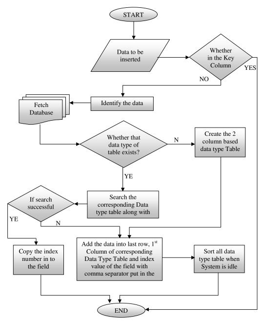
Figure 1: Flow Diagram of the Proposed Approach of Data De Duplication Technique.
