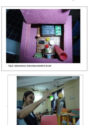
The amount of light needed to actuate the relay can be changed by changing the 220K potentiometer. Basically, any change to the potentiometer will have an effect on the voltage drop of the LDR, i.e. its sensitivity is adjustable depending on the available light intensity. Practical applications are shown in figure 5
