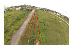
Figure. 1(e): Detected power-lines
