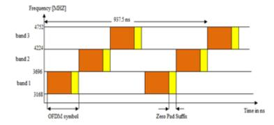
Figure 2. Example of time-frequency coding for MB-OFDM systems in the group1,  $TFC = \{1, 2, 3, 1, 2, 3, ...\}$
