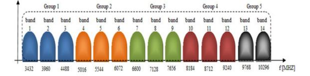
Figure 3. UWB spectrum bands in the MB-OFDM solution
