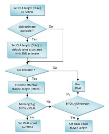
Figure 5. Process to dynamically evaluate the OLAL length based on the estimated SNR and CIR
