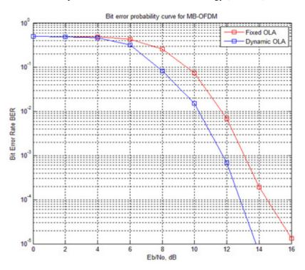
Figure 9. Comparison performance between fixed OLA and Dynamic OLA in the case of CM4 for 480 Mbit/s with TFC
