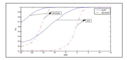
Figure 2. Pd versus SCR plots of GLRT (solid curves) and GCGLRT (dashed curves) receivers with Orthogonal DFCSTW Code set and STC for Pfa= $10^4$ , N = 8, Tx =4, Rx =4,  $\rho$  = 0.9, K = 64, v=0.5 parameter.
