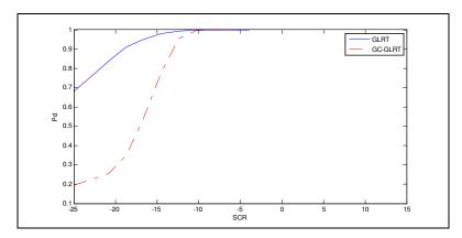
Figure 1. Pd versus SCR plots of GLRT (solid curves) and GCGLRT (dashed curves) receivers with Orthogonal DFCSTW Code set for Pfa= $10^{-4}$ , N = 8, Tx =4, Rx =4,  $\rho$  = 0.9, K = 64, v=0.5 parameter.
