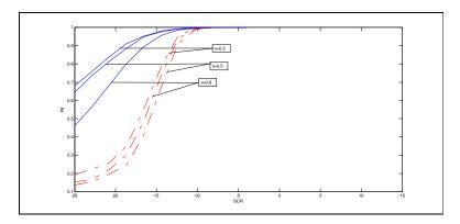
Figure 3. Pd versus SCR plots of GLRT (solid curves) and GCGLRT (dashed curves) receivers with Orthogonal DFCSTW Code set for Pfa= $10^4$ , N = 8, Tx =4, Rx =4,  $\rho$  = 0.9, K = 64, v=0.3, 0.5 and 0.8 as variable parameter.
