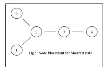
Initially five nodes are positioned in an open environment as shown in fig.3 for sensing the mechanism to route information depends totally on the path and its supportive algorithms. The direction of information transfer is calculated using the position of the node, protocols and the topology. Simulations are performed on NS2 and verification of results are generally discussed in sections to follow. The algorithm is as follows.
