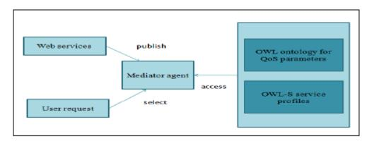
Figure 5.1 Modeling architecture for QoS based semantic WSS.
