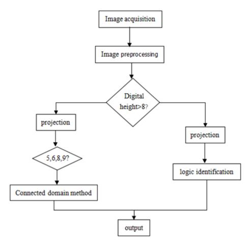
Figure 2 digital meter processing
