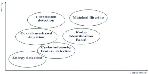
Figure 3. Sensing method complexity versus accuracy
