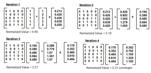
Figure 1: Example to Illustrate the Execution of the Power Iteration Method to Compute the Spectral Radius of a Network Graph
