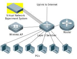
Figure 4. A experimental group with Virtual Network Experiment System
