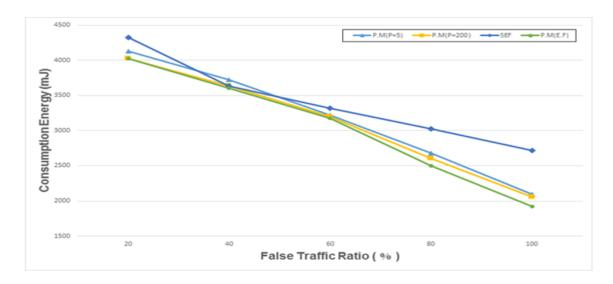
Figure 7. Energy consumption as a function of the FTR
