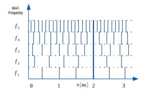
Fig. 1. Example demonstrates the process for solving the ToF based on measured phase. In each channel, there is a set of periodic solutions. The answer corresponds to the time when solutions for all the channels match [12].
