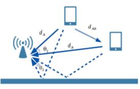
Fig. 2. Angle of direct path corresponds to the triangle with sides d<sub>A</sub>, d<sub>B</sub> and pAB. When signals from multipath components are tried, the angle does not fit this triangle [11].
