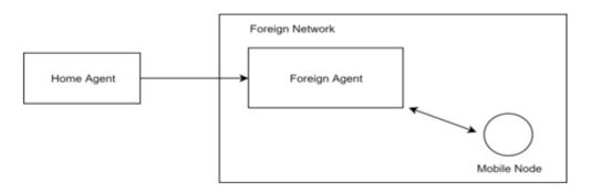
Figure 2. An Overhead View of IP Mobility Support for IPv4.
