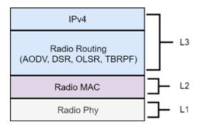
Figure 3. The First Three Layers of the MANET Radio Protocol Stack.
