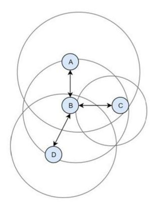
Figure 1. The Wireless Links Between Four MANET Nodes.
