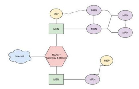
Figure 4. The MANET has two MBN connected to the MANET router over a wired interface (the thick line) as well as one or more MRN or MEP. The radio IP/radio protocol links are shown as thin lines and the links which only support radio protocol are shown as dotted lines.
